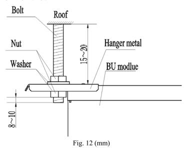
5) Adjusting the nuts position, so that the BU module should be level in front/back and left/right.
