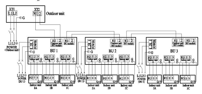
The "L1", "3" terminals are connected to the live wire, the "L2", "N(1)" terminals are connected to the neutral wire and the "2" terminal is connected to the transmission line.
